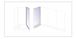
For installation on a wet floor, tiles or vinyl an extruded bottom profile must also be ordered. Product Code: 27221
